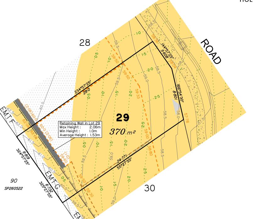
**LEGEND** Area of Cut Area of Fill Design Contours (0.50m Interval) Depth of Fill Contours (0.50m Interval) Proposed Retaining Wall (Height shown in brackets on lower side) (1.0) Proposed Earthworks Pad  $XX \cdot XX$ Proposed Earthworks Pad Design Level Top of Batter Toe of Batter Indicative Driveway Location
